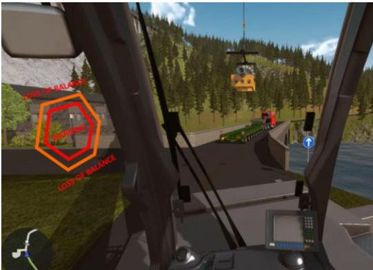
Figure 4: A warning on loss of balance. In this case, there is a loss of balance on the left side of the machine, thus the warning is presented on the left windshield<sup>4</sup>
