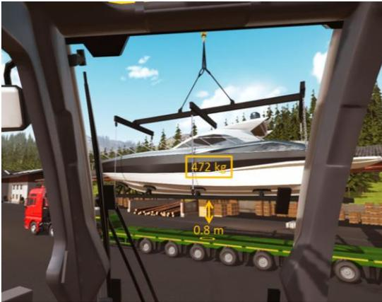
Figure 3: The information about the weight and the height of the lifted object is presented directly on the windshield<sup>4</sup>
