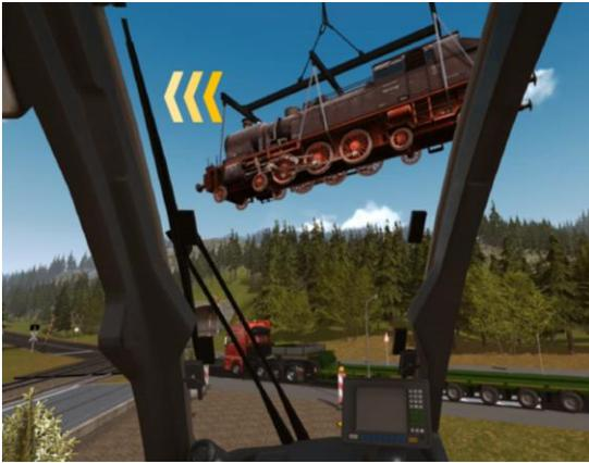
**Figure 5: Showing the direction where the lifted object should be moved when the destination is outside the operator's field of view<sup>5</sup>**
