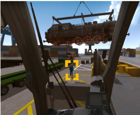
**Figure 6: A warning when there is a ground worker near the machine or the lifted object<sup>5</sup>**
