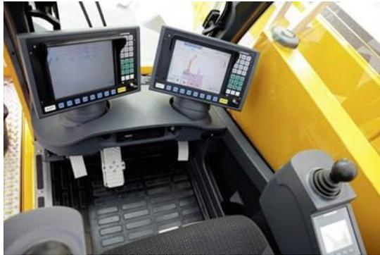
**Figure 1: An example of mobile crane's cabin. Operation-supporting information is presented using monitors on the dashboard<sup>2</sup>**
